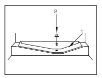
checkto ensure that no food particles have blocked the drain tube. The drain tube canbe cleared by pushing the special plastic plunger provided down the drain tube.
